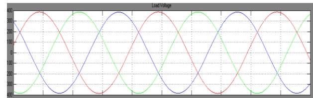
Figure 6.20 Load side voltage waveform of non linear load circuit with shunt active filter
