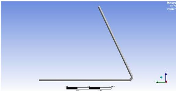
Fig. 5.21 65° Degree Elbow geometry import on ANSYS
