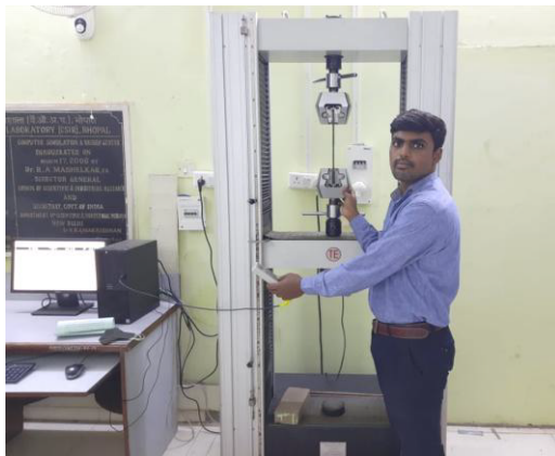
Fig: 4 Taking data during tensile testing with UTM machine
