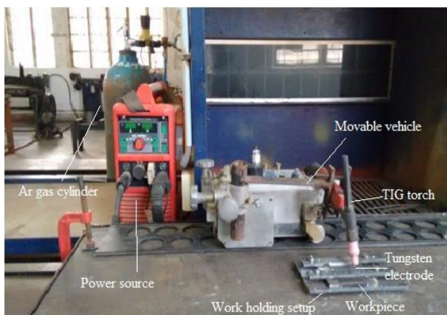
Fig.1 Experimental setup of TIG welding
