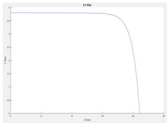
Fig. 8 I-V characteristics of PV module
