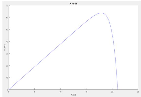
Fig. 7 P-V characteristics of PV module
