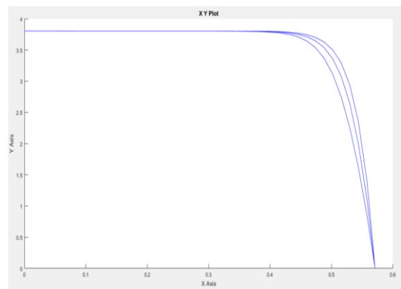
Fig. 14 I-V characteristics for effect of varying  $R_s$
