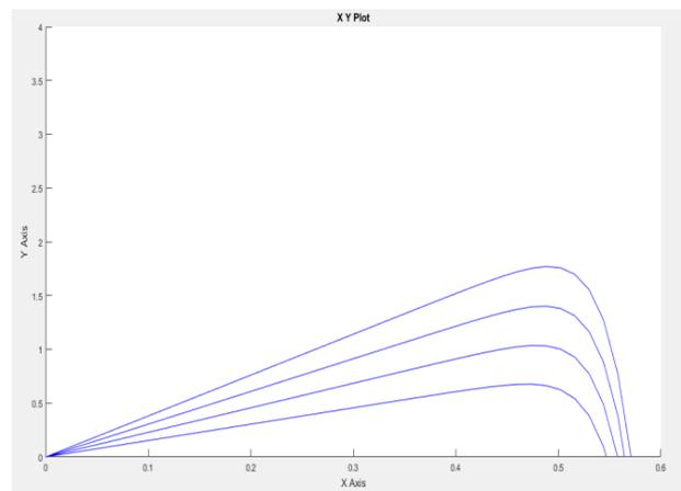
Fig. 19 P-V characteristics for effect of varying solar radiation
