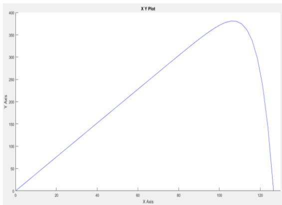
Fig. 11 P-V characteristics of PV Array
