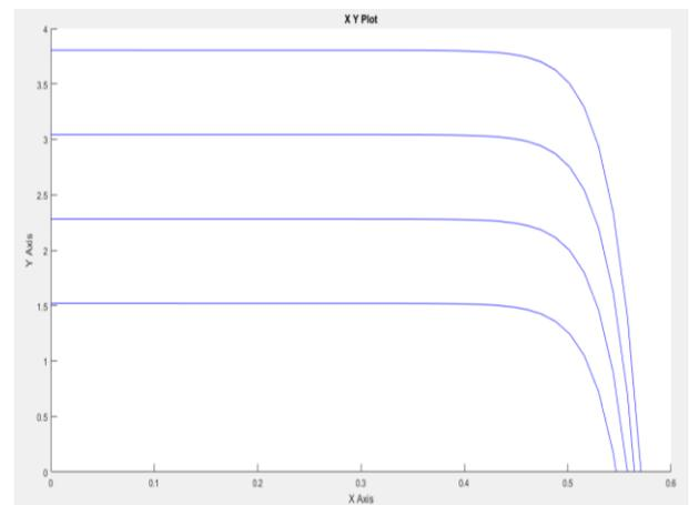
Fig. 20 I-V characteristics for effect of varying solar radiation
