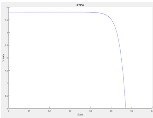
Fig. 5 I-V characteristics of PV Cell
