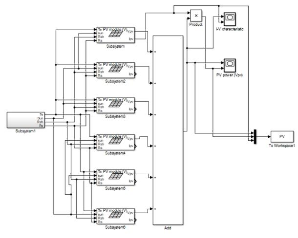
Fig. 9 Simulation model of PV Array
