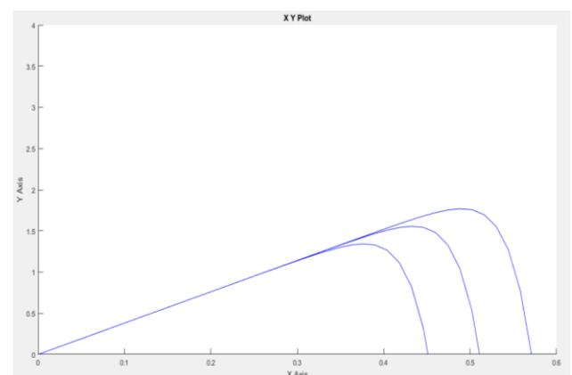
Fig. 25 P-V characteristics for effect of varying  $I_s$
