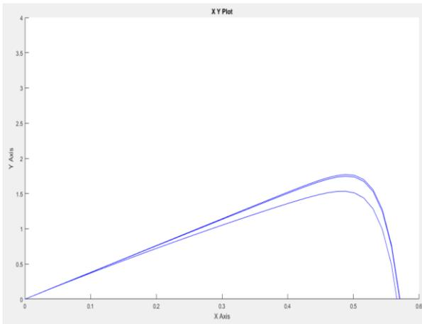
Fig. 16 P-V characteristics for effect of varying  $R_{sh}$
