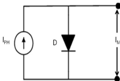
Figure 2. 1-D Ideal model for a Solar cell
