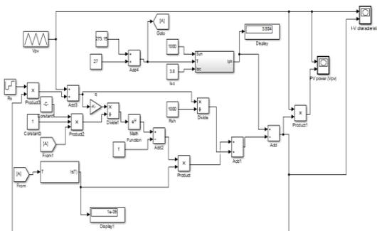
Fig. 12 Simulation model of PV array for effect of variation of series resistance
