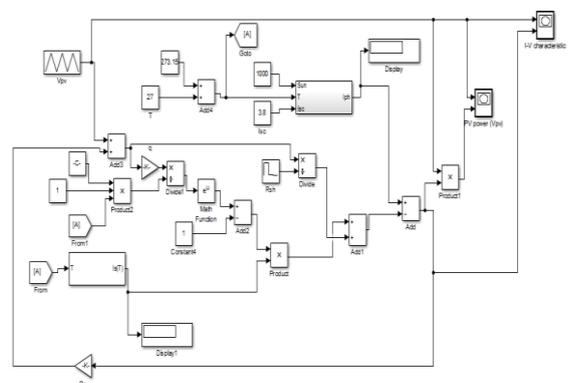
Fig. 15 Simulation model of PV array for effect of variation of shunt resistance
