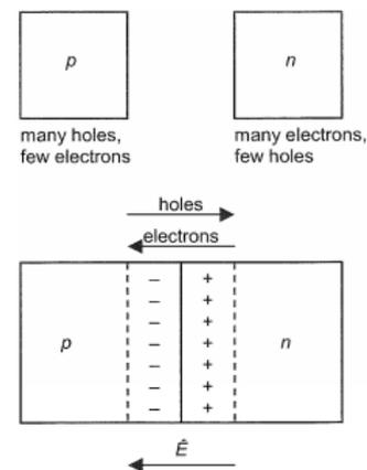
Figure 1 P-N Junction of Different Part of The Semiconductor
