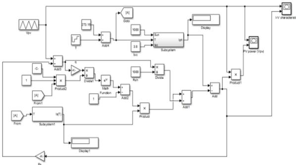
Fig. 21 Simulation model for effect of varying temperature
