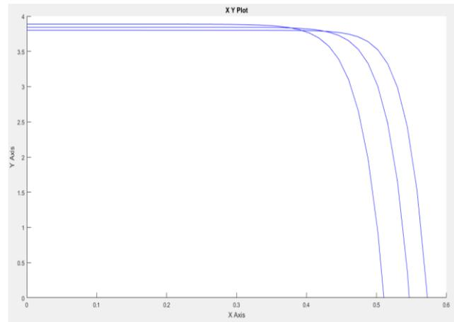
Fig. 23 I-V characteristics for effect of varying temperature
