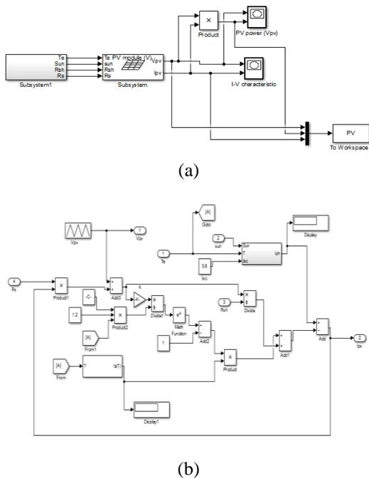
Fig. 6 (a) Simulation model of PV module (b) subsystem configuration
