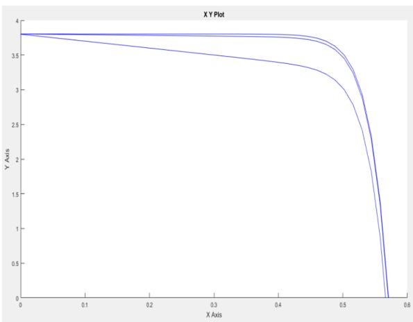
Fig. 17 I-V characteristics for effect of varying  $R_{sh}$
