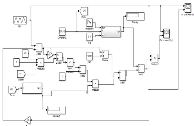
Fig. 18 Simulation model for effect of varying solar radiation
