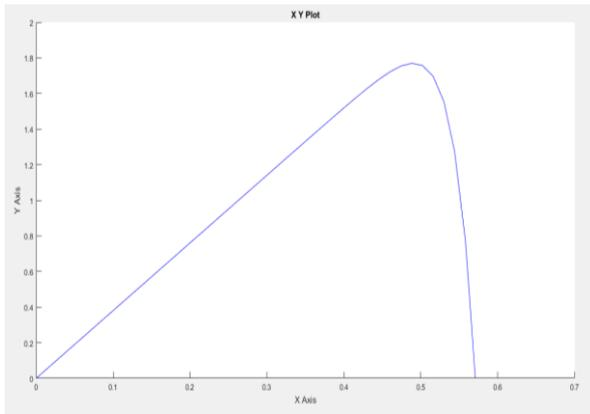
Fig. 4 P-V characteristics of PV Cell
