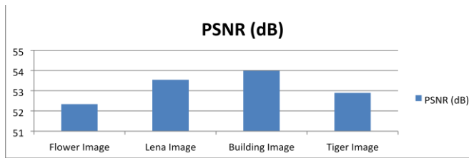
Figure 5.9: PSNR of the Different Image with 50 characters and .jpg format
