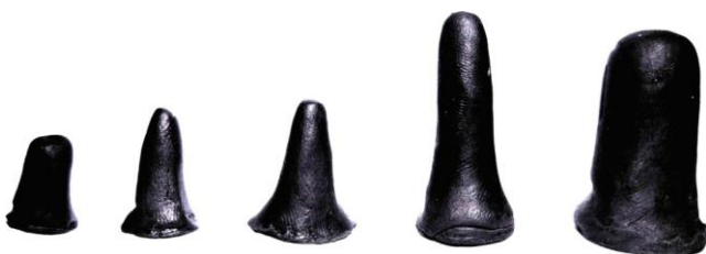
Figure 6: Epoxy compound statues at 65% solidification of total solidification time
