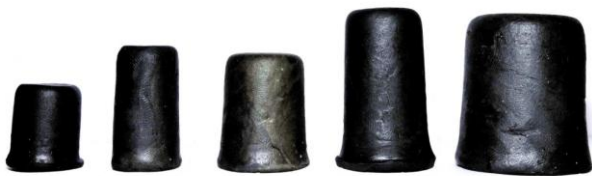
Figure 5: Epoxy compound statues at 40% solidification of total solidification time
