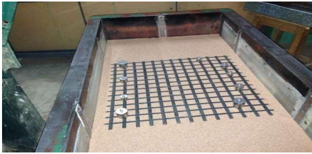
Figure 1: Placement of geogrid during experiment
