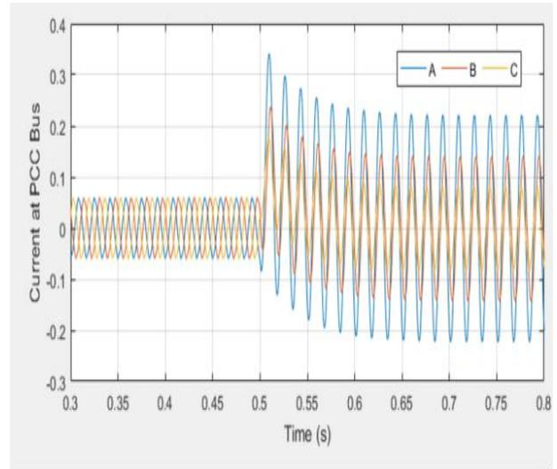
**Figure 5:** Current waveform at PCC Bus due to line-ground fault in Grid
