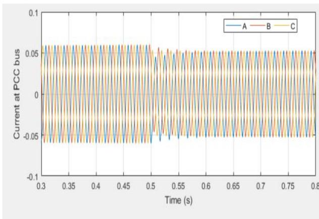
**Figure 4:** Current waveform at PCC Bus due to PP fault in PV array.
