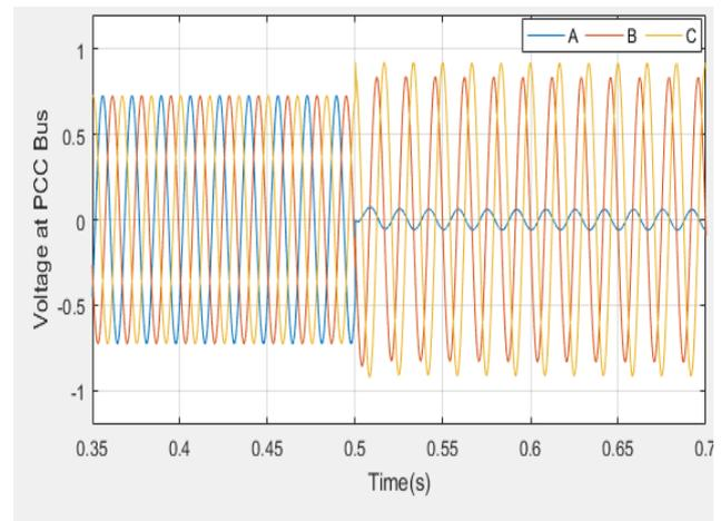
**Figure 6:** Voltage waveform at PCC Bus due to line-ground fault in Grid
