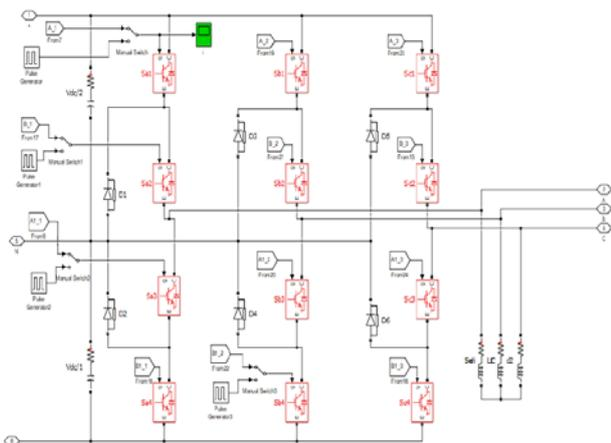
**Figure 5:** A simulink model of 5-level Neutral point clamped (NPC) inverter configuration.
