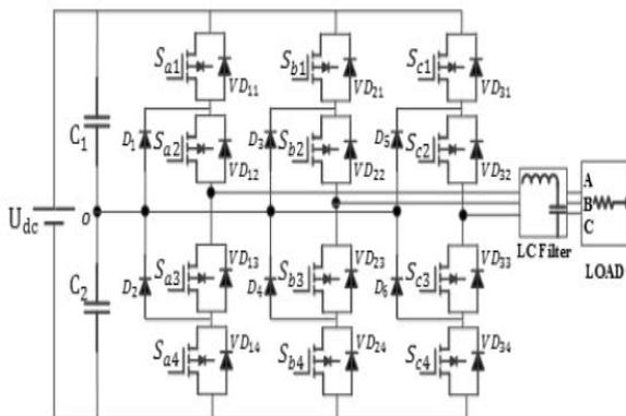
Figure 2: Circuit diagram of the NPC multi-level inverter.
