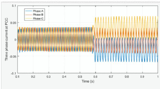
**Figure 8:** Three-phase current signal at PCC bus B1 due to the short circuited operation of Sa1.
