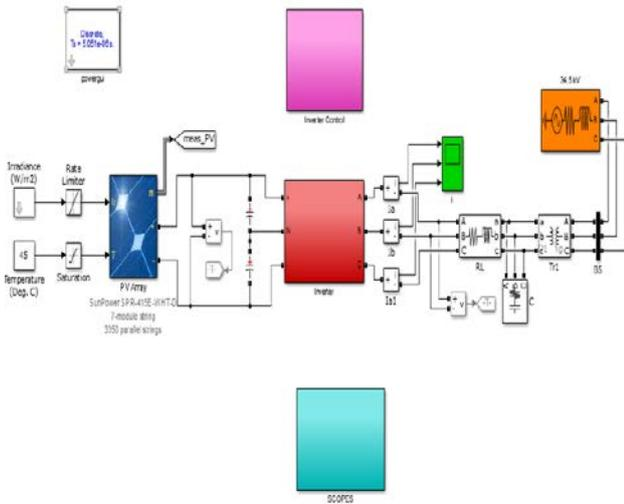
**Figure 4:** Grid connected PV system Simulink model.
