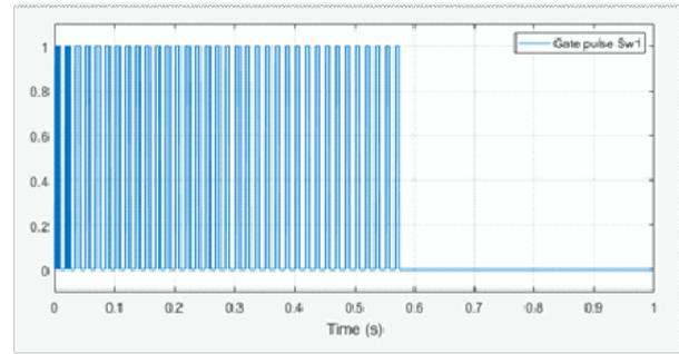
**Figure 6:** Gate pulse with switch Sa1 short-circuited at t=0.57s
