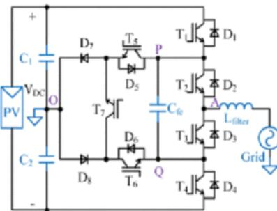
Figure 1: Neutral-point clamped (NPC).
