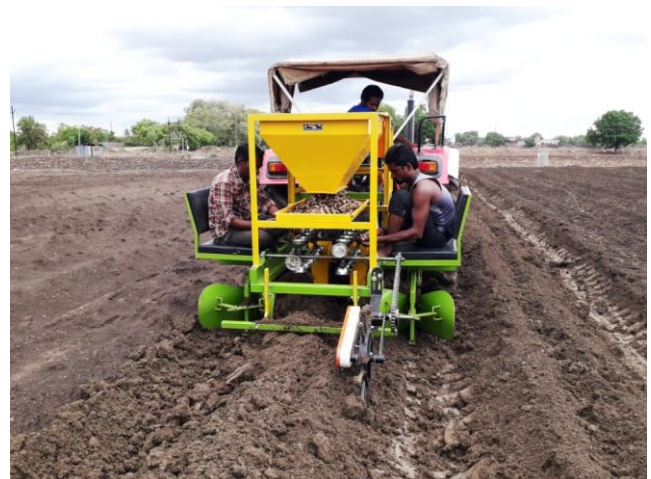
Fig 1: Tractor drawn turmeric planter
