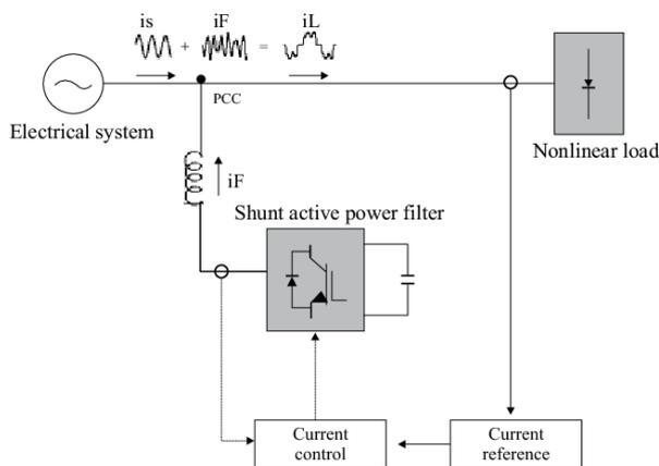
Fig. 1.2 Schematic Diagram of a Shunt active filter.
