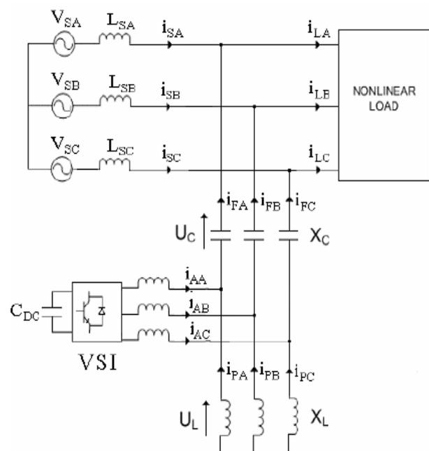
Fig.1.1. Simplified Electrical Diagram of a HAPF
