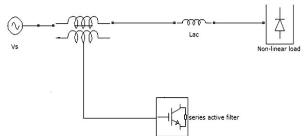
Fig.1.3 Schematic diagram of series active filter
