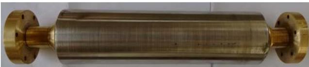
Fig.4 Photographic view of Regenerator
