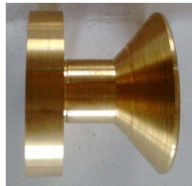
Fig.5 (b) Bottom flange of Pulse tube
