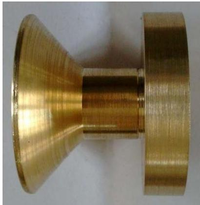
Fig.3 (b) Bottom flange of Regenerator
