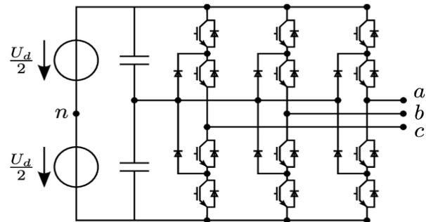
Figure 1: Neutral-Point-Clamped (NPC).
