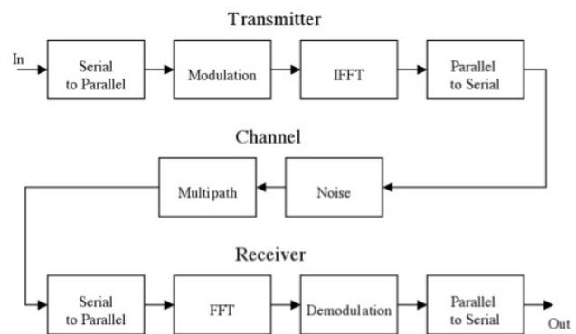
Fig.2.1 OFDM Transmitter and Receiver
