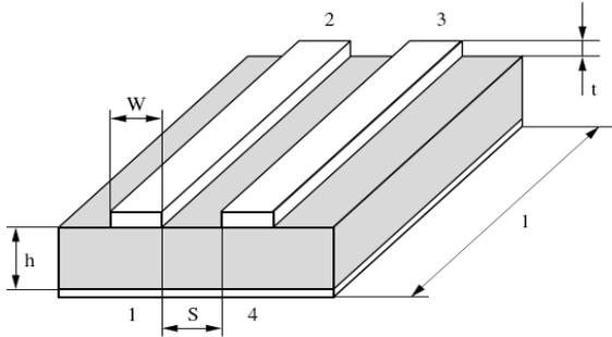
Figure.1 Geometry of the microstripline.
