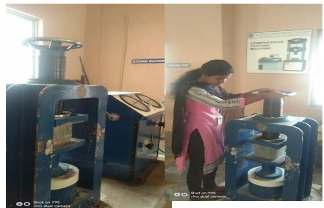
Fig 4: Compressive Strength Testing
