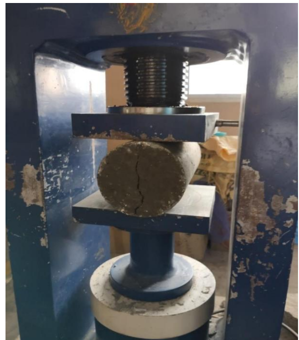
Fig. 2 Split tensile strength by using CTM
