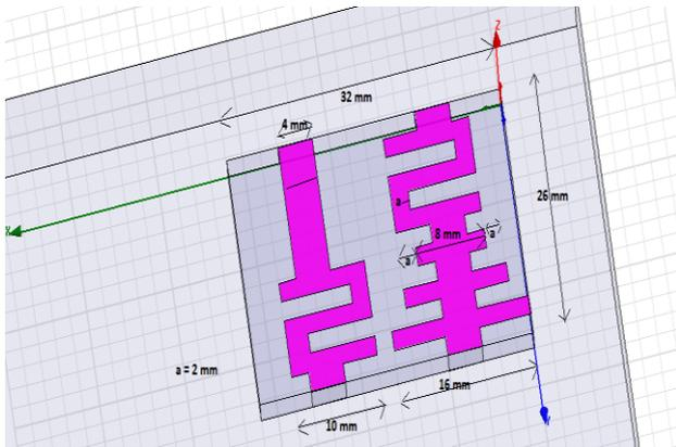
**Figure 4:** Top view of the 2<sup>nd</sup> Design of Reduced Cross Coupled Line Directional Coupler Model.
