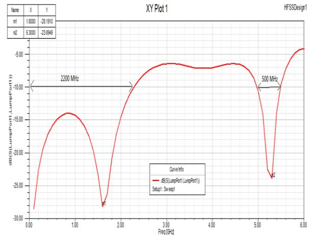
**Figure 10:** Return loss of simulation result for Design 2
