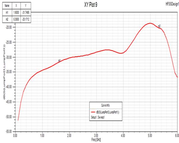
**Figure 18:** Coupling Factor Coefficient  $S_{31}$  of simulation result for Design 3.
