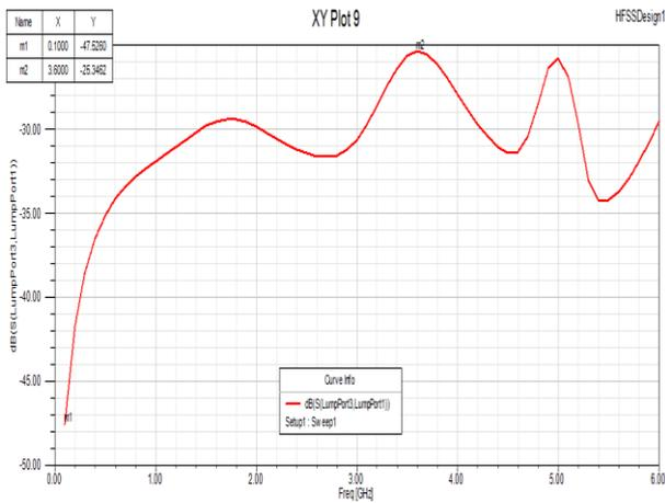
**Figure 8:** Coupling Factor Coefficient  $S_{31}$  of simulation result for Design 1.
