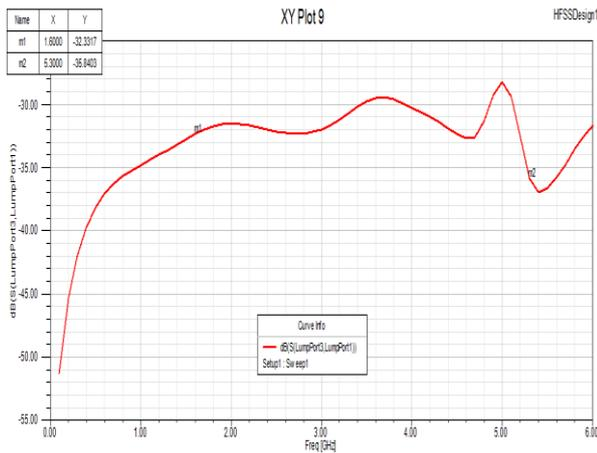
**Figure 13:** Coupling Factor Coefficient  $S_{31}$  of simulation result for Design 2
