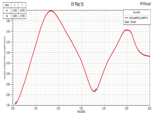
**Figure 7:** Insertion Loss of simulation result for Design 1
