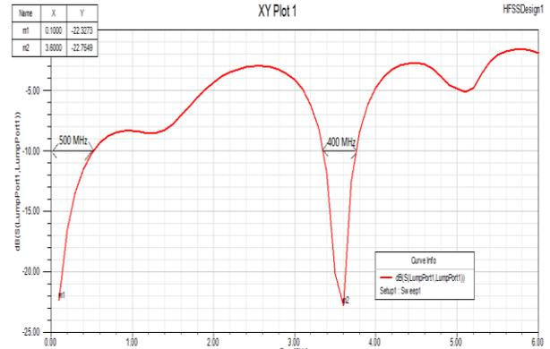
**Figure 5:** Return loss of simulation result for Design 1.
