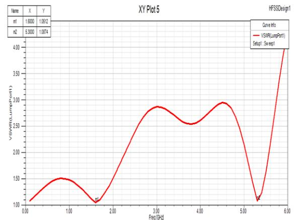
**Figure 16:** VSWR of simulation result of 3<sup>rd</sup> Design hybrid line directional coupler model.
