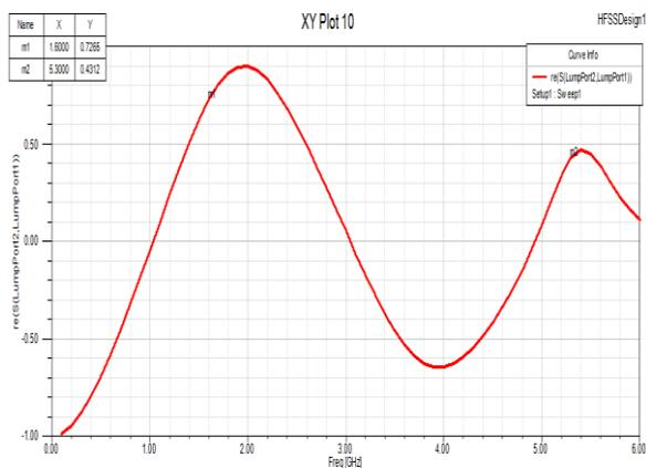
**Figure 17:** Insertion Loss of simulation result for Design 3.
