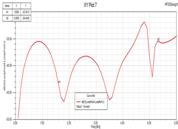
**Figure 14:** Isolation Coefficient  $S_{41}$  of simulation result for Design 2.
