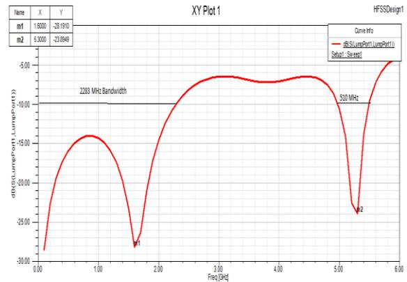
**Figure 15:** Return loss for 3<sup>rd</sup> Design.
