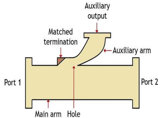
**Figure 1:** Two Ports Directional Coupler.
