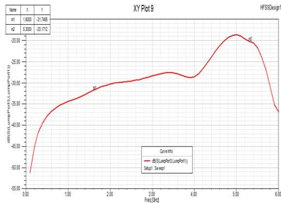
**Figure 19:** Isolation Coefficient  $S_{41}$  of simulation result for Design 3.
