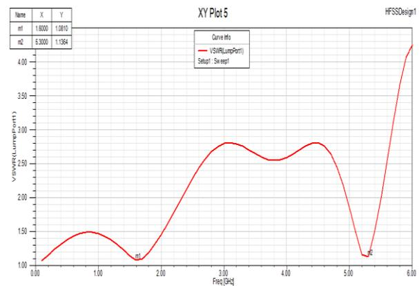
**Figure 11:** VSWR of simulation result of 2<sup>nd</sup> Design at Port 1
