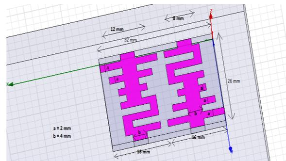
**Figure 2:** Top View of Cross Couple Line Directional Coupler for Design 1.
