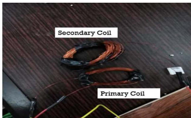
Fig.11. Wireless Power Transfer Setup
