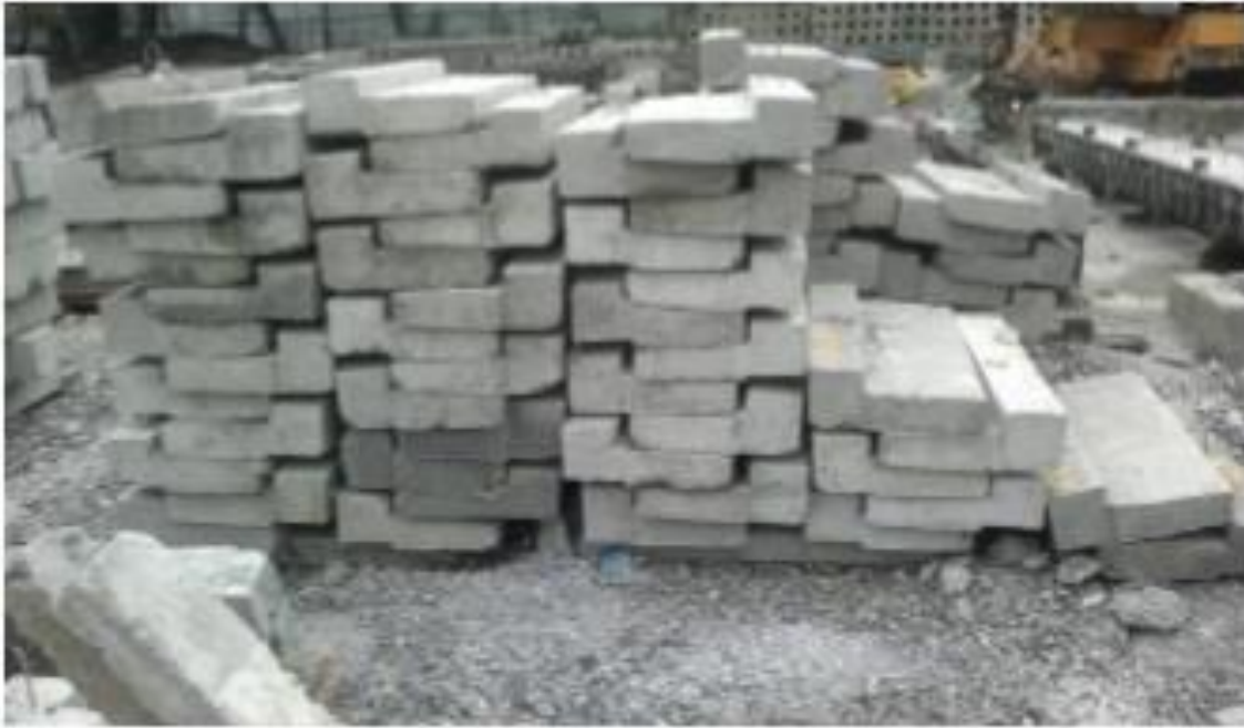
Figure 4.11 Sample of Prefabricated Lintel and Chajja
