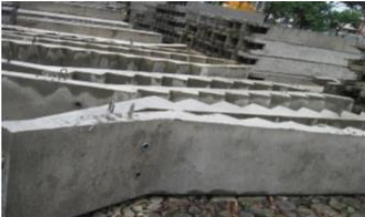
Figure 4.10 Sample of Prefabricated Stair Case
