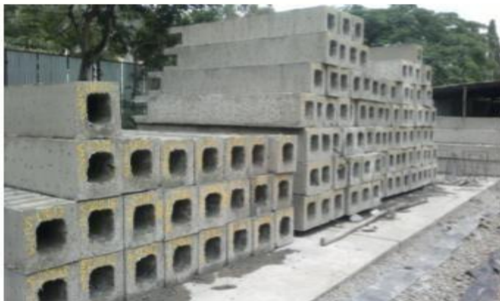
Figure 4.6 Sample of Prefabricated Column
