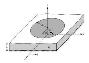
Figure 1. Basic circular patch antenna.
