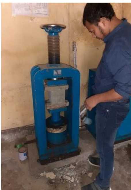
Figure 4.7 Compressive Strength Test
