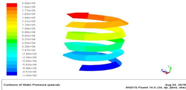
Fig. 4.3.1 Pressure contours for Triangular Cross-sections
