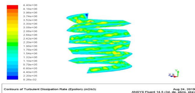
Fig. 4.3.4 Contours of Turbulent Dissipation Rate for Triangular Cross-sections
