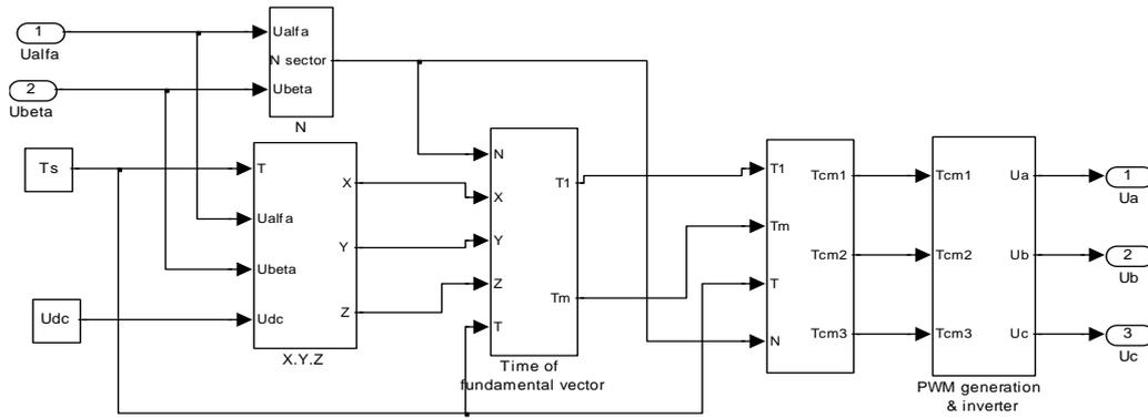
Fig.3 Simulink model of SVPWM inverter
