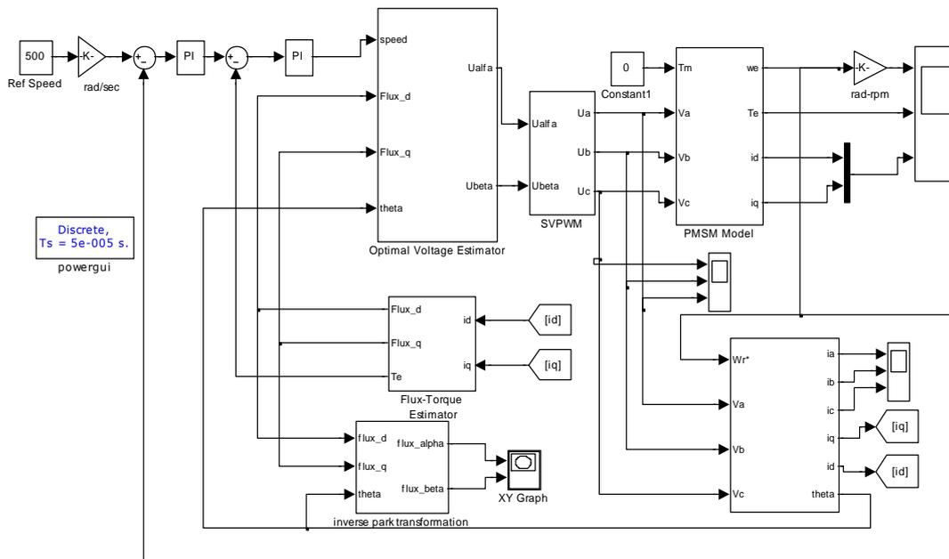
Fig 4 Simulink model of direct torque control scheme of PMSM drive
