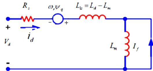
Fig .1(a) Equivalent Circuit of PMSM(d - axis)
