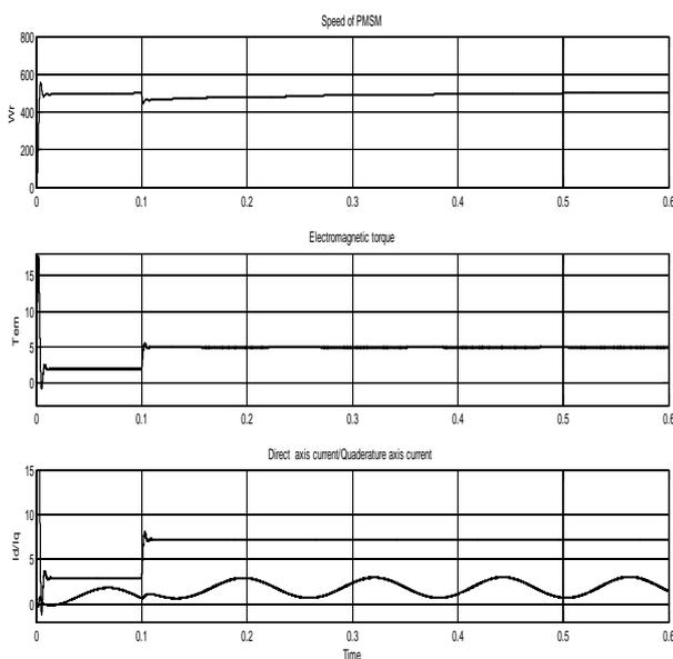
Fig-5 speed pmsm(  $\omega_r$  in rpm ), electromagnetic torque( In Nm), current  $I_d$ ,  $I_q$  (in ampere) of (for  $\omega_r=500$  at  $t=0.1$ sec,  $T_L= 2$  to  $5$ Nm)
