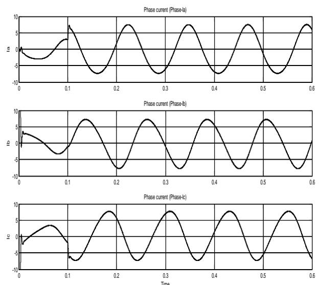
Fig-6 Three phase motor current( in ampere) (for  $\omega_r=500$ rpm at  $t=0.1$ sec,  $T_L=2$  to  $5$ Nm)
