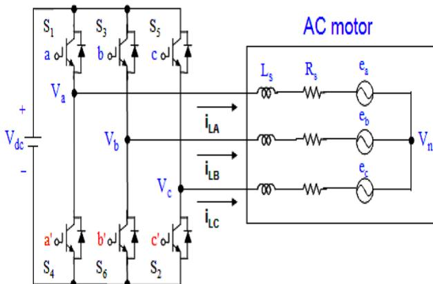
Fig.2 Bridge inverter
