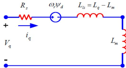
Fig .1(b) Equivalent Circuit of PMSM (q- axis)
