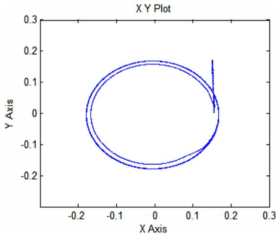
Fig 8 - Flux trajectory between  $\alpha$  – axis flux (x axis) and  $\beta$  – axis Flux (y axis)
