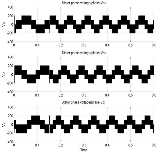
Fig-7 Three phase stator voltage( in volt) (for  $\omega_r=500$  at  $t=0.1$ sec,  $T_L=2$  to  $5$ Nm)
