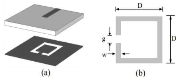
Figure 1: DGS resonator configuration
