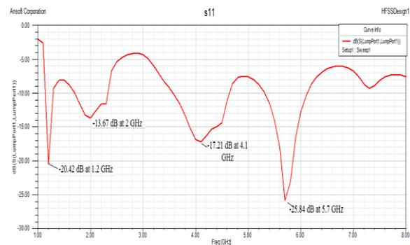
Figure.8: Return loss of simulation result for Design 2 With FR-4 substrate.
