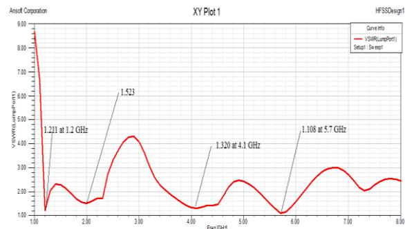
Figure.9: VSWR of simulation result for Design 2 With FR-4 substrate.
