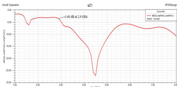
Figure.7:Insertion Loss of simulation result for Design 1 With FR-4 substrate.
