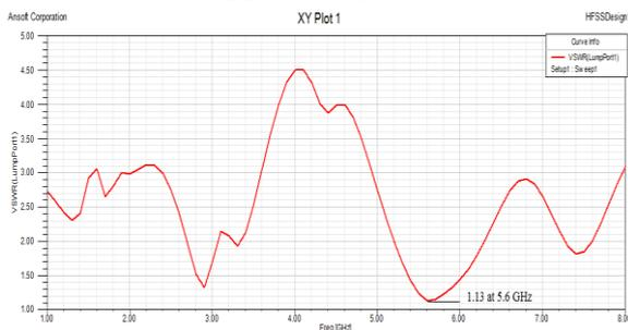
Figure.6:VSWR of simulation result for Design 1 With FR-4 substrate.
