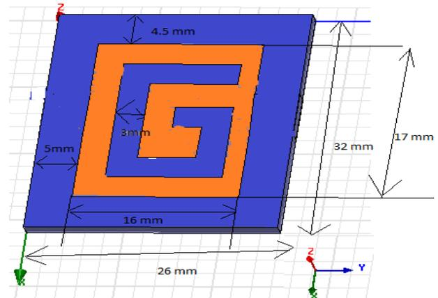
Figure.4 Bottom view of 2nd Design ground plane.
