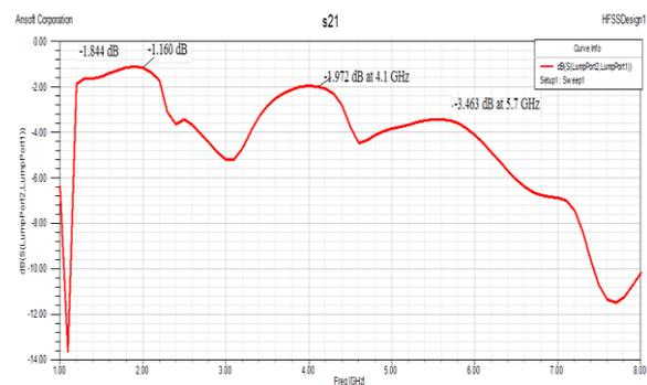
Figure.10: Insertion Loss of simulation result for Design 2 With FR-4 substrate.
