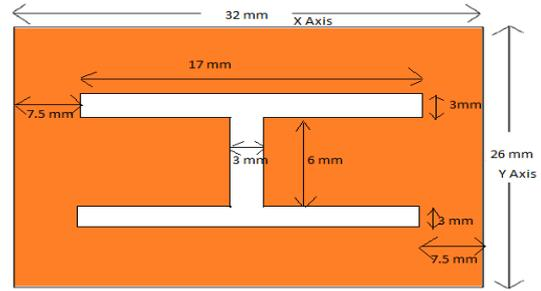
Figure.3 Bottom view of 1st Design ground plane.
