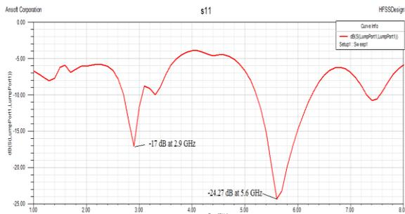
Figure.5:Return loss of simulation result for Design 1 With FR-4 substrate.
