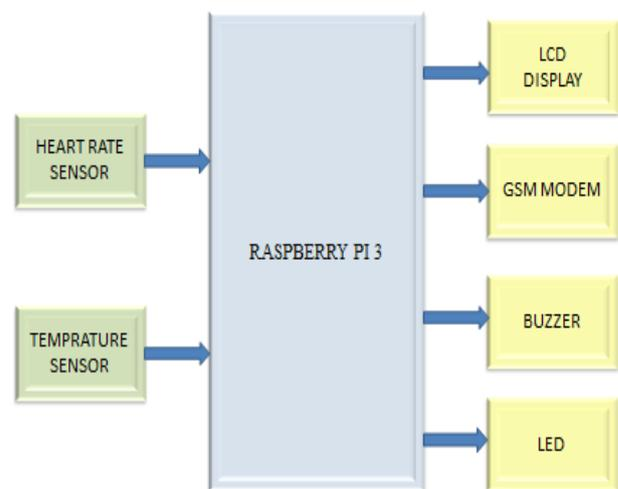
The proposed IOT based health monitoring system works with the help of Raspberry Pi 3 as the Central Processing unit and the basic input devices that is used in this are heart rate sensor, temperature sensor. And the output devices that is used are LCD 16x2 with male header pin with blue backlight display, GSM SIM800 modem module with SMA antenna, piezoelectric buzzer and LEDs[2].
