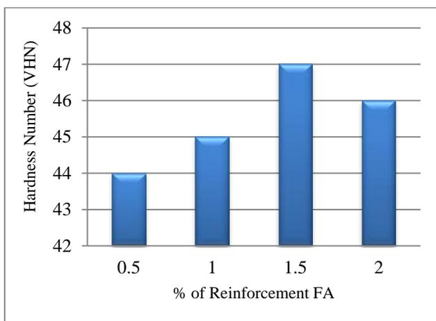
**Fig. 3: Hardness P/M samples of Mg/FA nanocomposites**
