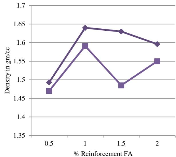
Fig 2: Density trend of Mg/FA before and after sintering
