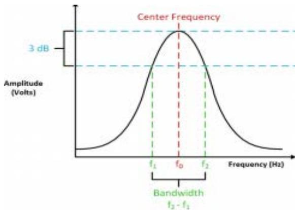
Figure 4: Frequency response of bandpass filter
