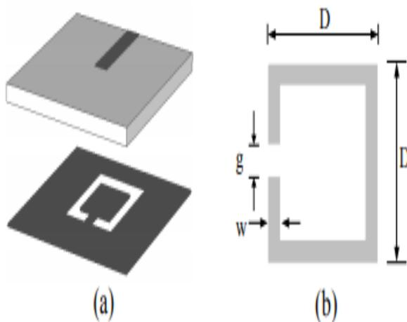
Figure 2: DGS resonator configuration
