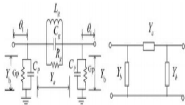
Figure 1 : RLC circuit modeling of unit DGS cell
