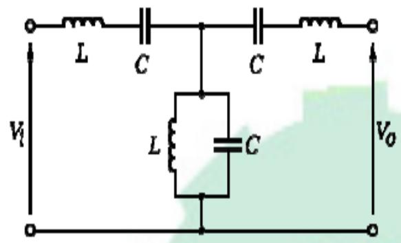
Figure 3: Band pass filter circuit
