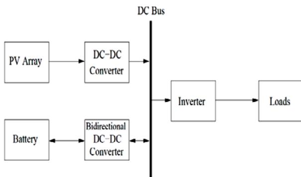
Fig. 2.1 Standalone PV systems with battery load.
