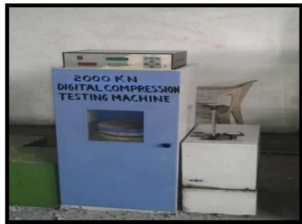
Fig.3.11. Compressive Strength Testing Machine
