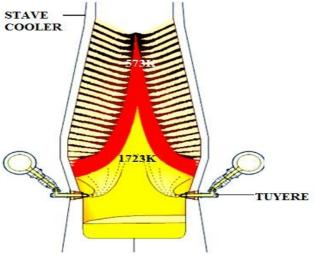
Thermal Zone of Blast Furnace
