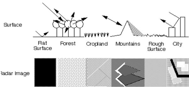
Figure 2.1 Imaging different types of surface with radar [12]
