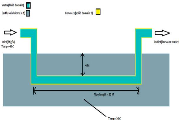
The pipe is contacting with the surrounding underground environment makes the temperature of the pipe surface is almost or similar as temperature of the ground at particular depth. This temperature is usually lower than ambient temperature. In this way, heat is transferred to the surrounding soil by means of convection in the air tunnel to the pipe wall and conduction from the pipe wall to the surrounding soil.
