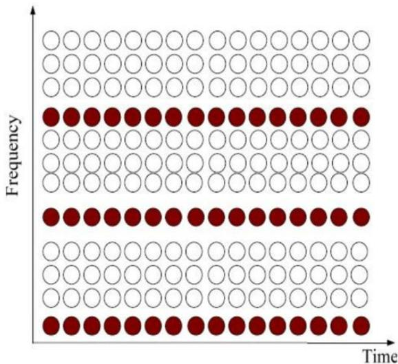
Fig. 2 Pilot Arrangement in OFDM System.
