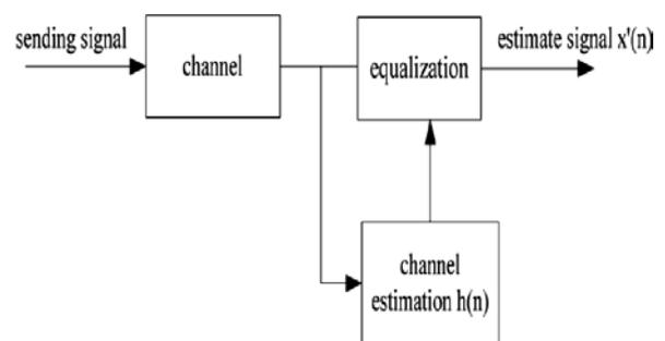
Fig. 1 Block diagram of channel estimation.
