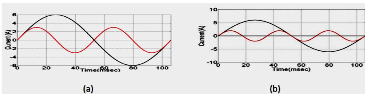
Figure 2.1 A sinusoidal waveform with fundamental frequency and its harmonic (a) 50Hz,(b) 100Hz.
