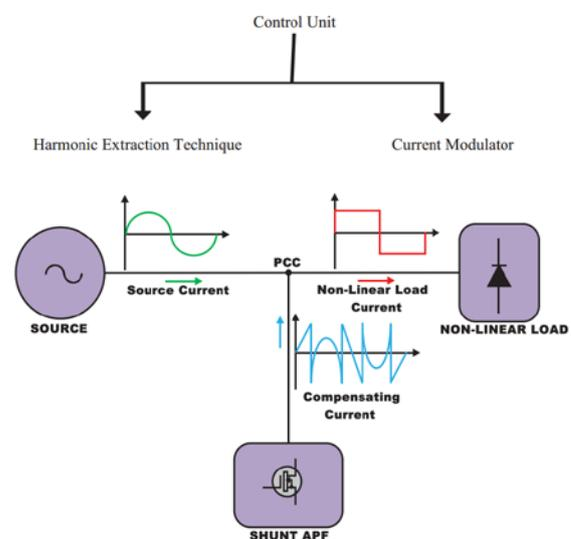
Figure 1.1 Shunt Active Power Filter.
