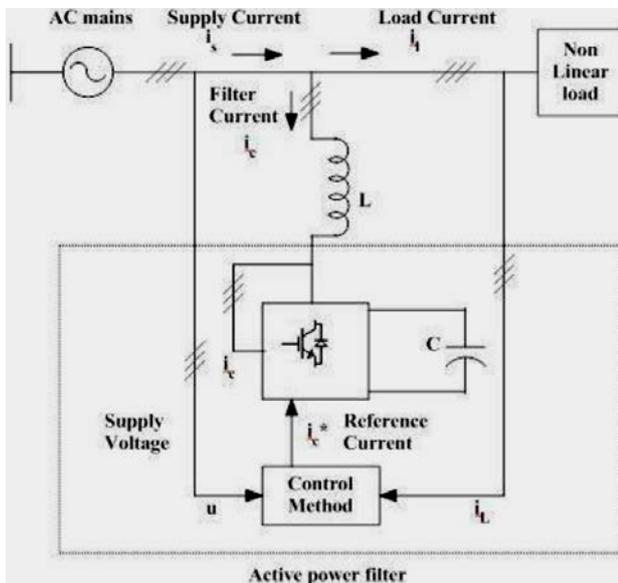
Figure 2.2 Schematic Diagram of shunt active power filter.
