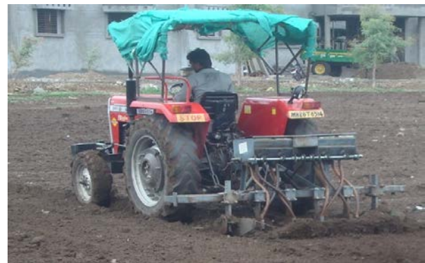
Plot 3: Demonstration planting soybean crop with BBF planter (Tractor and BBF planter)
