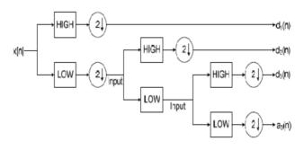
Fig. 2 Block diagram of the 2-level DWT scheme
