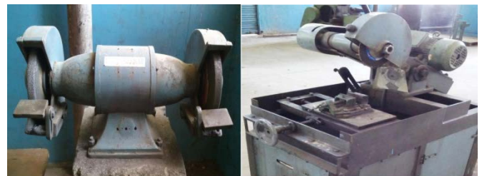
Fig. 4.1 Grinding Machine and Abrasive Cutting Machine
