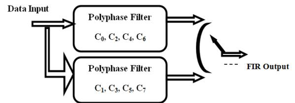
Fig.3: polyphase decomposition for interpolation filters
