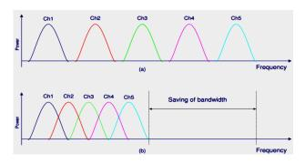
Figure 2.1 Comparison between conventional FDM and OFDM.
