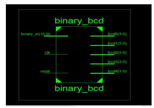
Fig.2 Block Diagram of 16 bit Binary coded decimal Converter
