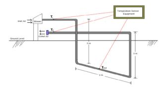
Schematic Representation of Experimental Set up
