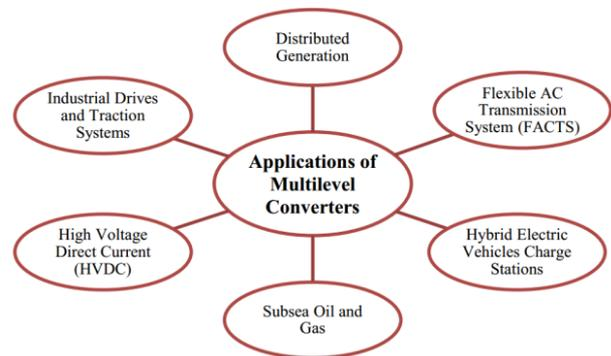
Fig. 1.1: Applications of Multilevel Converters.
