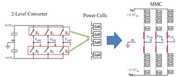
Fig. 1.2 Modular Multilevel Converter conceptual realization
