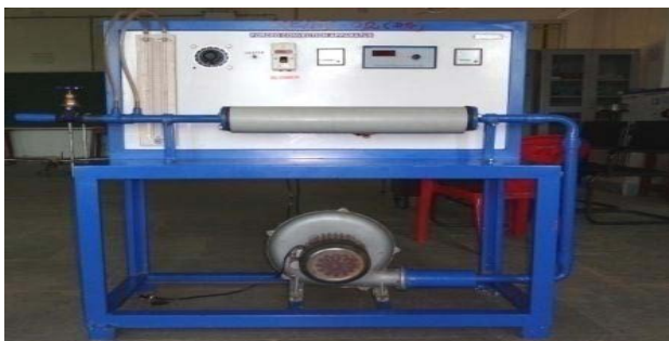
Fig.2 Experimental set up of Forced convection Apparatus
