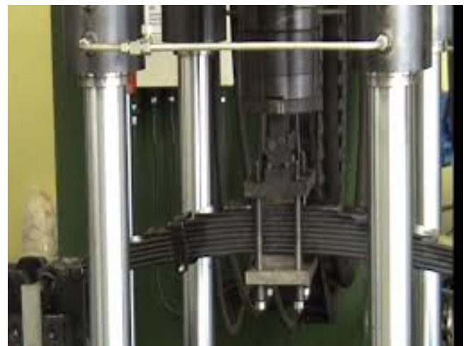
Fig 1: Leaf Spring under loading condition
