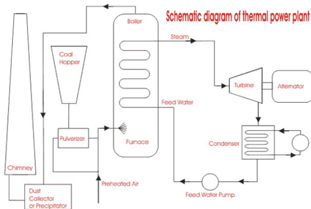
Figure 1.2 Thermal power plant
