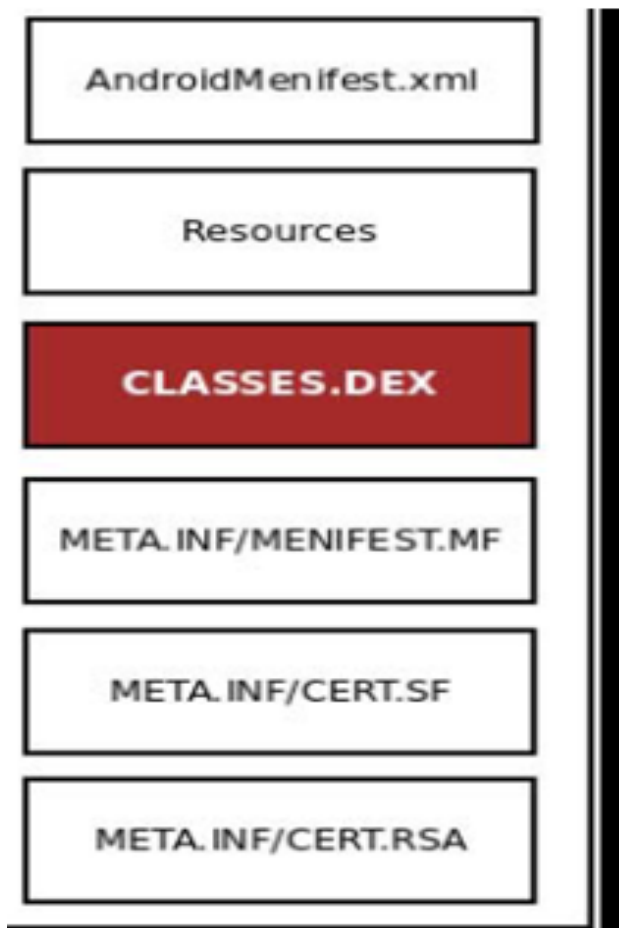
Figure 2. Android Package File format [6]
