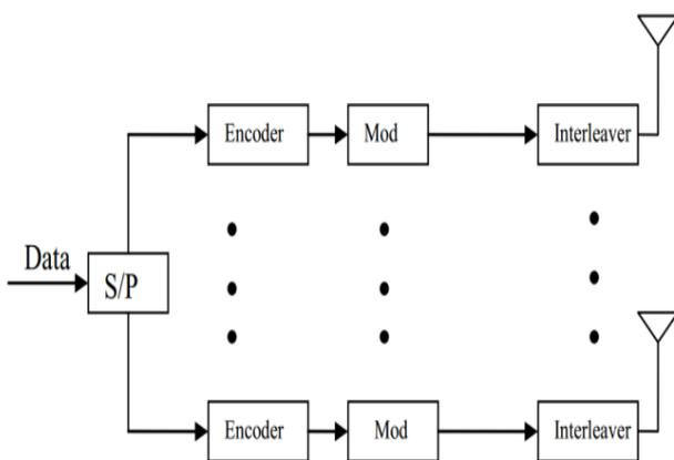
Fig. 1.3: H-BLAST Transmitter
