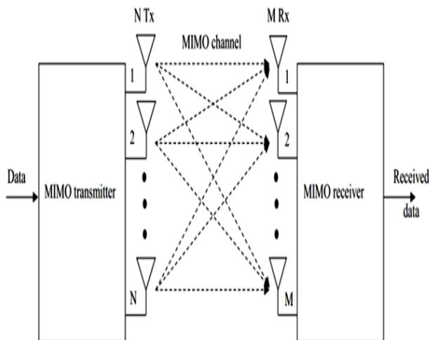
Fig. 1.1 Schematic of the generic MIMO system employing N transmitter antennas and M receiver antennas
