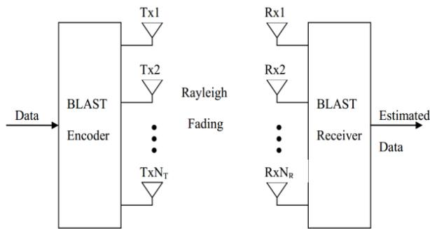
Fig. 1.2: A Typical BLAST Architecture
