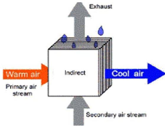
Figure 1.2 Indirect Evaporative Cooling[1]
