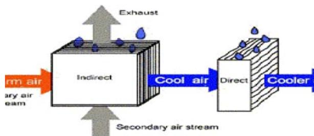
Figure 1.3 Direct and indirect Evaporative Cooling[1]
