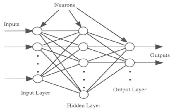
Figure 5. Feed forward distributed time delay network
