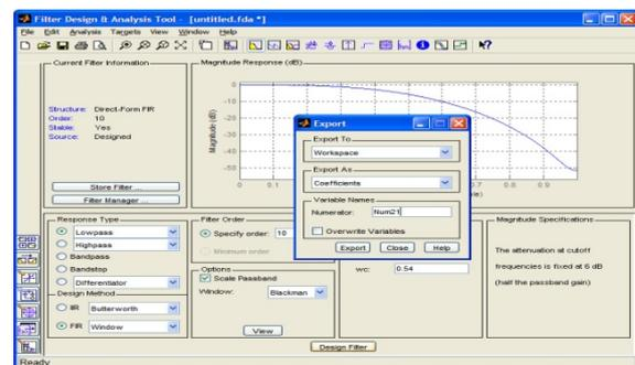
Figure 12. Filter coefficients by FDA tool
