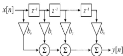
Figure 1. Simple low pass FIR filter
