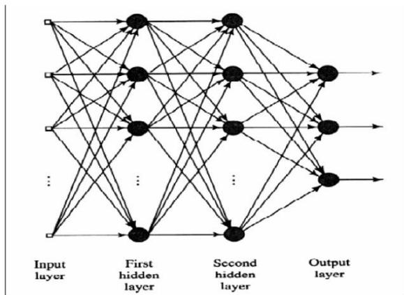
Figure 3. Feed forward back propagation network
